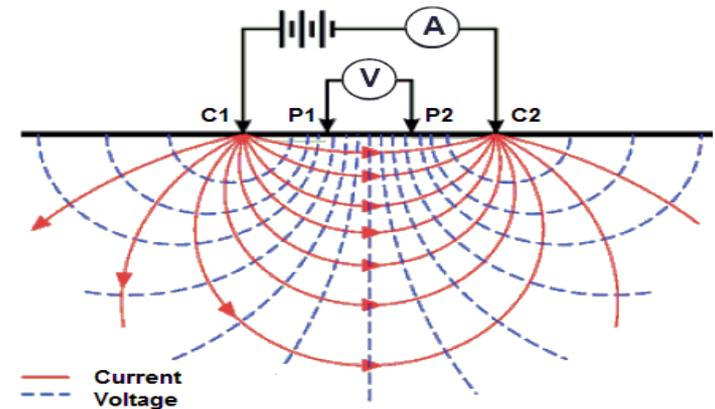
**Four-electrode resistivity Method**
