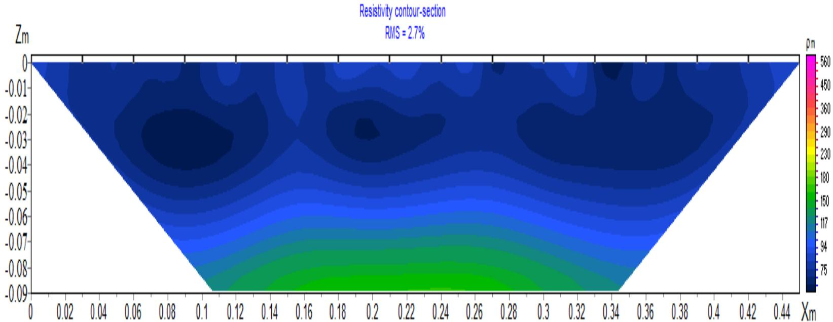
2D Resistivity sections of a water-filled container
