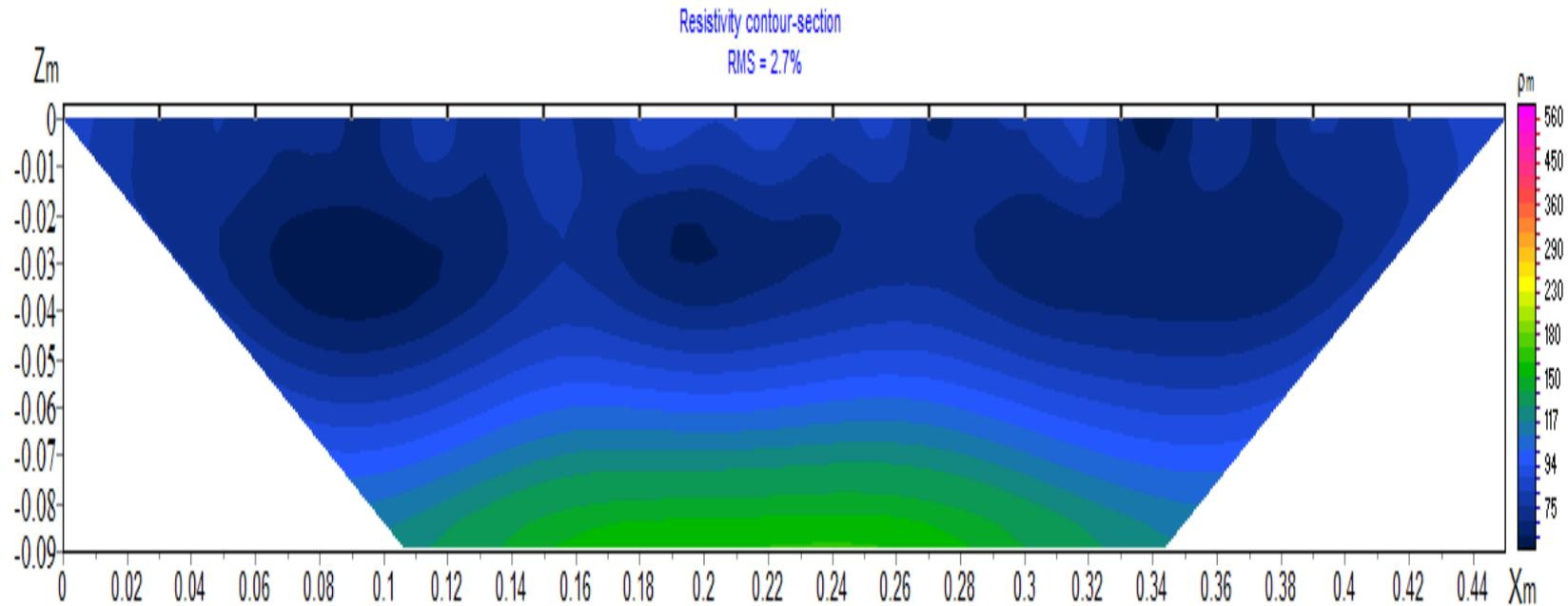
2D Resistivity sections of a water-filled container
